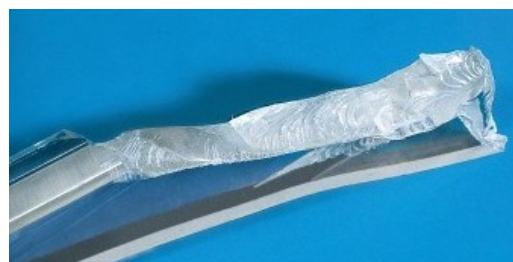
Fig. 2: Brittle fracture on a part made of hydrolytically degraded material.
